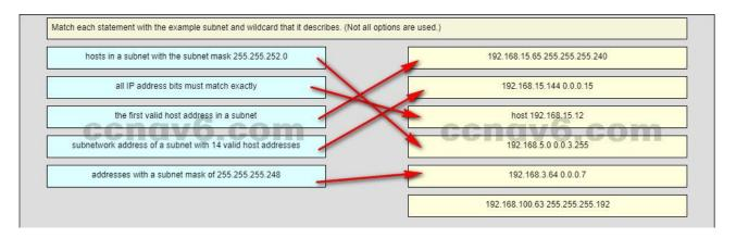
Converting the wildcard mask 0.0.3.255 to binary and subtracting it from 255.255.255.255 yields a subnet mask of 255.255.252.0.
